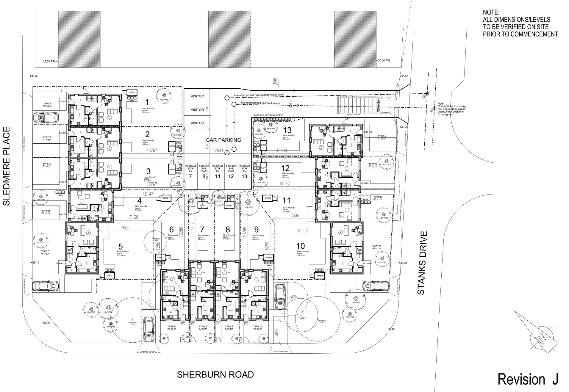
PROPOSED SITE LAYOUT SCALE - 1:100 @ A0 - 1:200 @ A2
